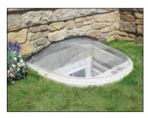
Limits the accumulation of snow, leaves and debris. Constructed of polycarbonate, this high impact cover is UV-resistant and designed for durability and long-life. Dome is designed to withstand a 40 PSF load and is supplied with quick release hold-down clips.
